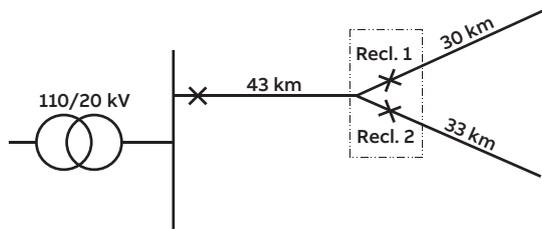
point was further chosen in such a way that 65% of the mean power of the feeder was located upstream of the station and thus out of reach of faults arising on the feeder section downstream of the recloser station. The mean powers of the line sections downstream of the reclosers amount to about 18% and about 17% of the mean power of the feeder.
