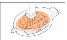
Fig 1. Flow pattern in the melt in a spout tapping furnace fitted with an ArcSave stirrer
