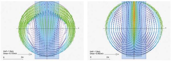
Fig 2. Melt flow velocity vectors simulated in a 100 ton spout tap EAF  $\ensuremath{^{[2]}}$
