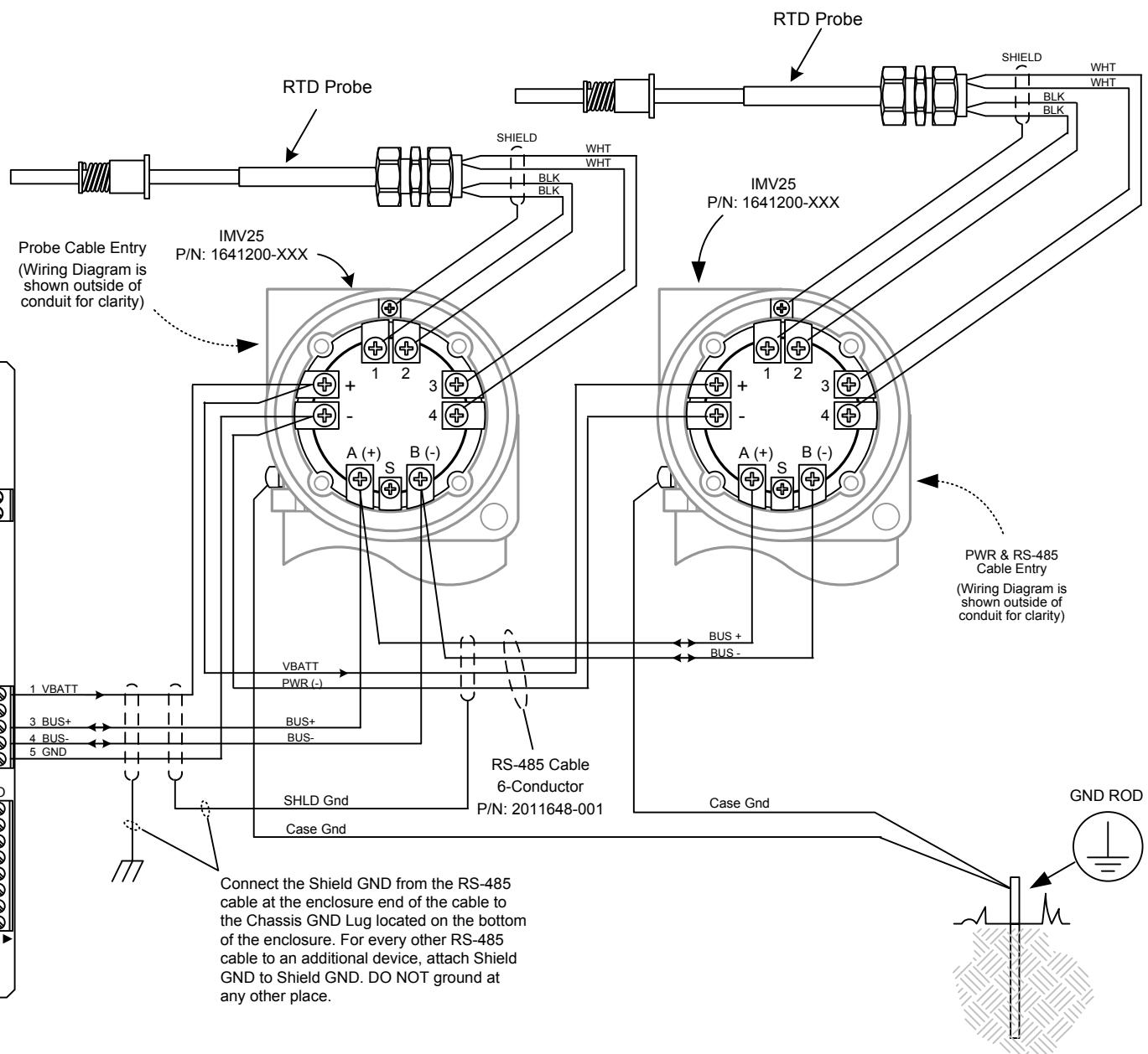
3. The RS-485 bus must be wired in a daisy-chain configuration. Star configurations are not allowed.
