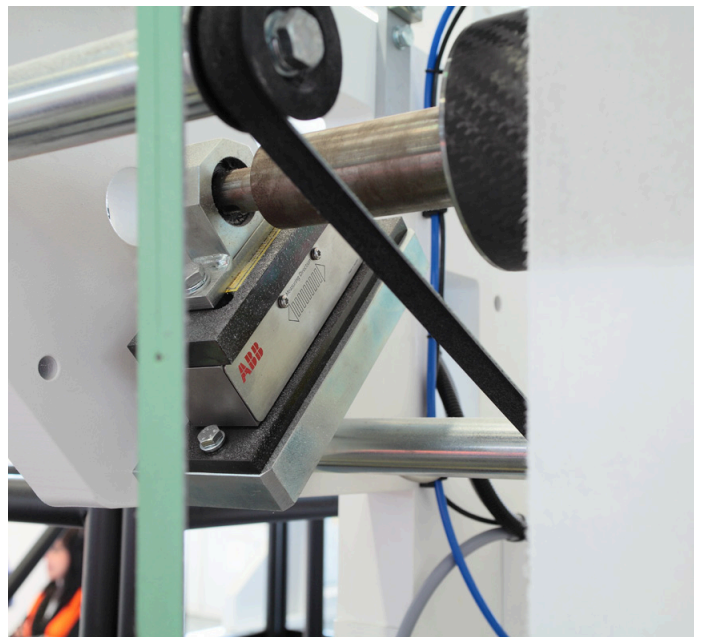
Mini-PillowBlock load cells (Mini-PBT) installed in tissue converting machinery from PCMC Italy. In instances where the force component in the measuring direction is insufficient or non-existent, the Mini Series PillowBlocks can be mounted at an angle.
