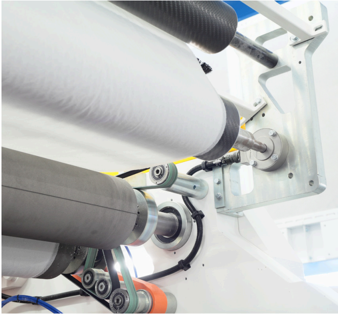
Pressductor Radial Tensiometers Load Cells (PRT load cells) installed in tissue converting machinery from PCMC Italy. No matter what the wrap angle is or where the measurement roll is located on the machine, the PRT load cell is simply rotated to pick up the ideal measurement force component.
