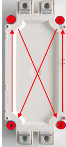
05 Tightening sequence to mount the module to the heat sink
