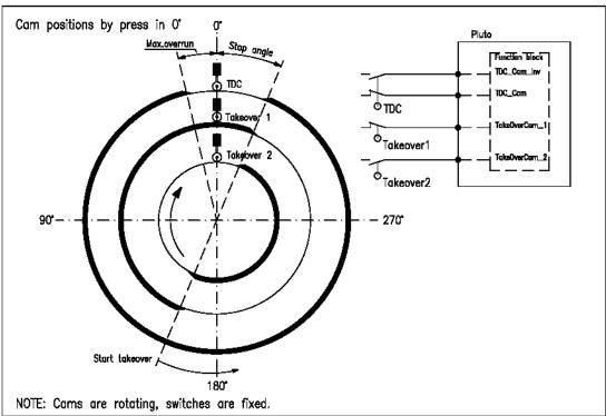
Example with three cam switches where the takeover is doubled. The two takeover cams have opposite function in order to achieve diversity.
