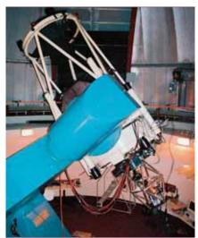
transmittance reaches over 60 percent (30 percent per CCD) at 500 nm, thanks to the use of a detector with 90 percent quantum efficiency. This is a value that is unmatched by any other spectrometer. The cameras are cooled with liquid nitrogen, enabling a very low readout noise (3 electrons) and hence a high sensitivity. This instrument can literally count photons.
