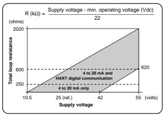
The total loop resistance is the sum of the resistance of all elements of the loop, including wiring, conditioning resistor, safety barriers and additional indicators (excluding the equivalent resistance of the transmitter).
