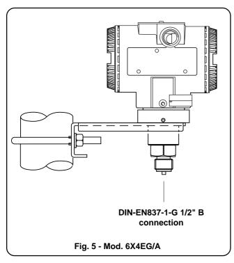
WARNING - For installation in Hazardous Areas, i.e. areas with dangerous concentrations of e.g. gases or dusts that may explode if ignited, the installation must be carried out in accordance with relative standards either EN 60079-14 or IEC 79-14 and/or with local authority regulations, for the relevant type of protection adopted. Together with safety information here and after enclosed see also the Addendum for "Ex Safety" aspects which is part of this instruction manual.
