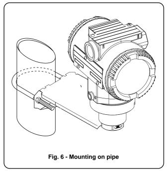
CAUTION - Proper location of the transmitter with respect to the process pipe will depend upon the service for which the instrument is used. Care should be exercised to identify correct process connections.
