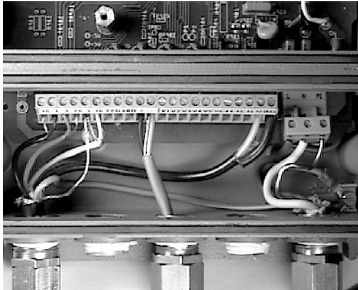
**FIGURE 2-6. RECOMMENDED CUSTOMER CONNECTION BOX WIRING**
