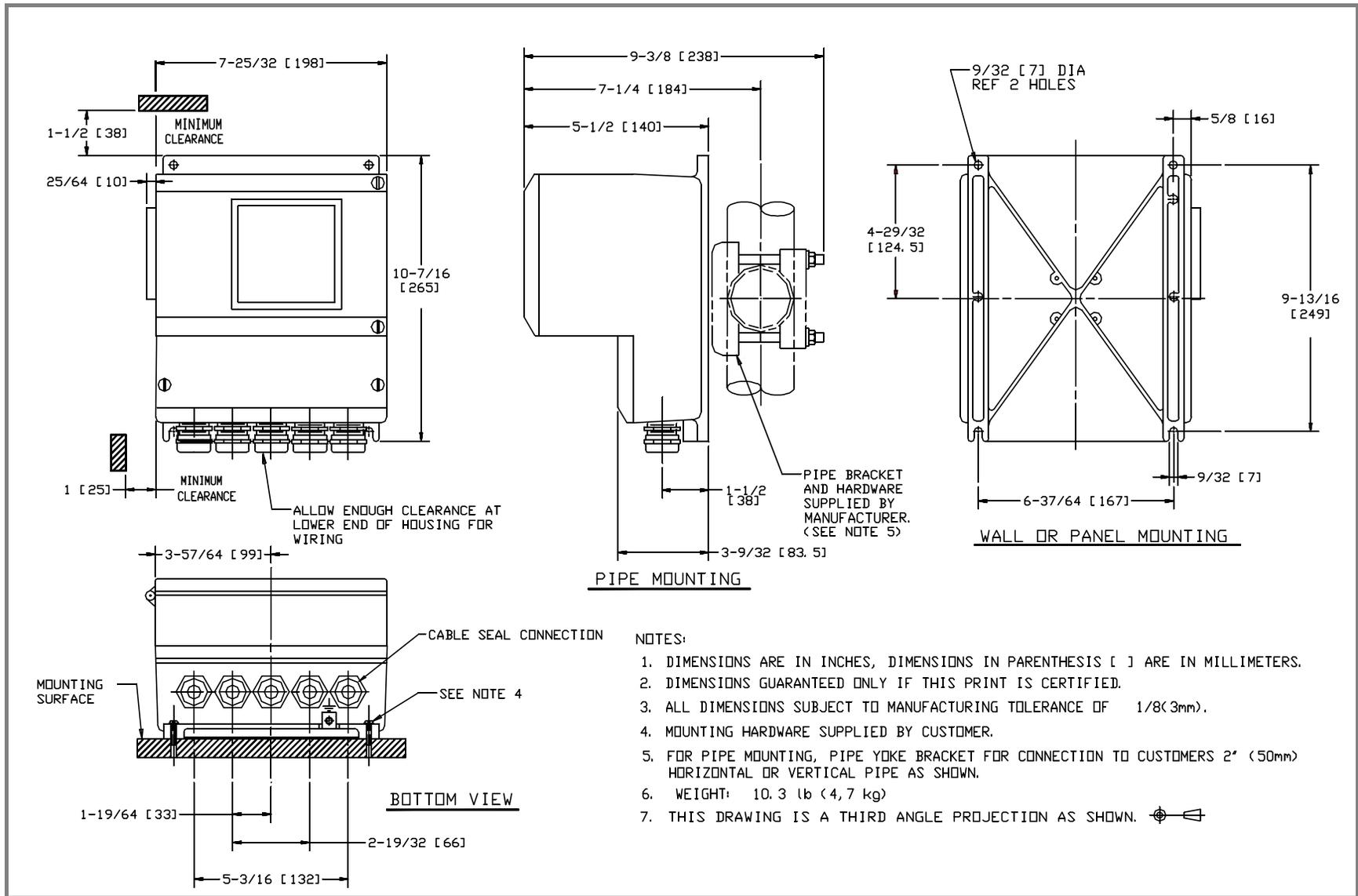
**FIGURE 2-4. OUTLINE DIMENSIONS, REMOTELY MOUNTED 50XM1000D SIGNAL CONVERTER WITH HINGED COVER & CABLE SEAL CONNECTIONS**
