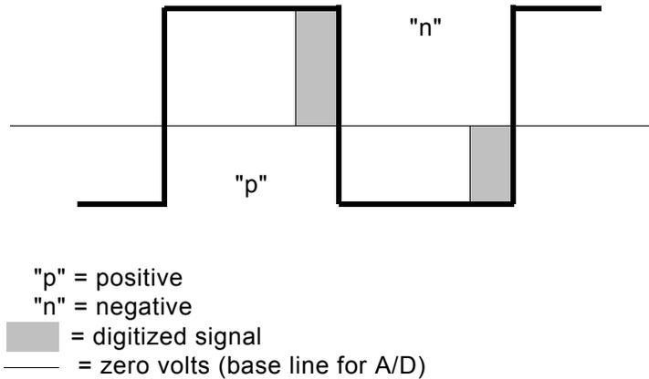
Note the wave form is not perfectly centered about the zero volt reference. This is typically due to DC voltages present at the electrodes and the fact that their influence on signal cannot be completely eliminated.
