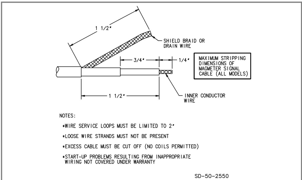
**FIGURE 2-5. RECOMMENDED WIRE PREPARATION**
