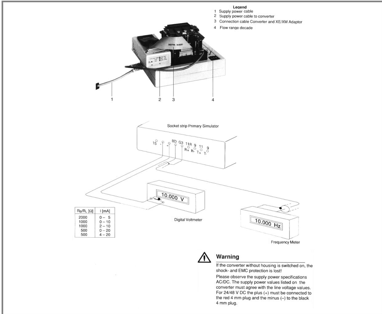
FIGURE 5-3. TEST WIRING USING 55XC4000 SIGNAL SIMULATOR
