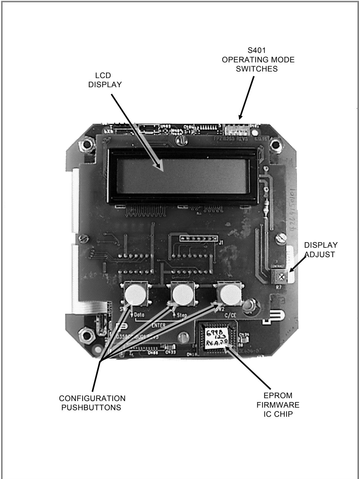
FIGURE 1-5. SIGNAL CONVERTER MODULE, TOP VIEW
