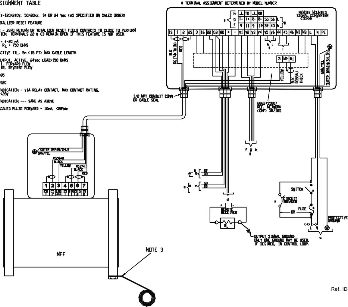
FIGURE 2-14. INTERCONNECTION WIRING FOR MODELS MFE & MFF WITH REMOTELY MOUNTED SIGNAL CONVERTER
