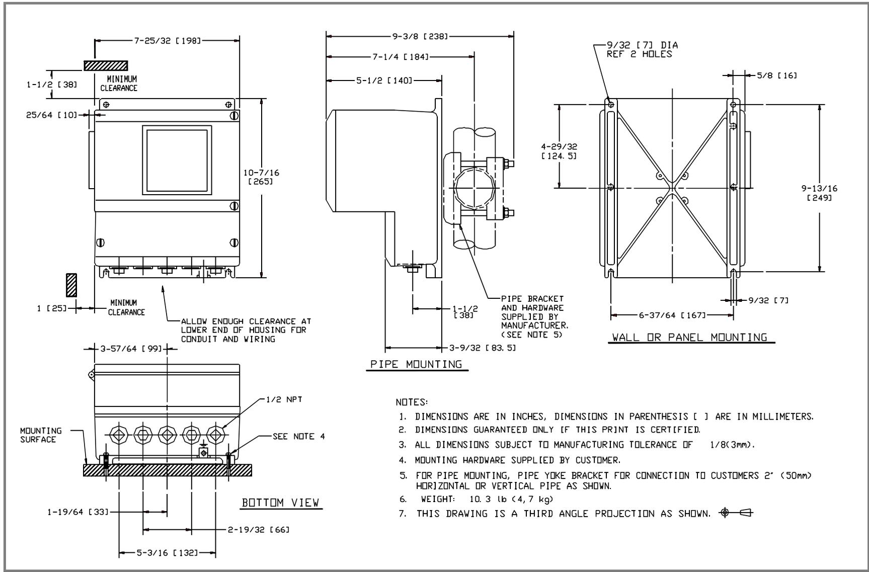
**FIGURE 2-3. OUTLINE DIMENSIONS, REMOTELY MOUNTED 50XM1000D SIGNAL CONVERTER WITH HINGED COVER & 1/2 INCH NPT CONNECTIONS**
