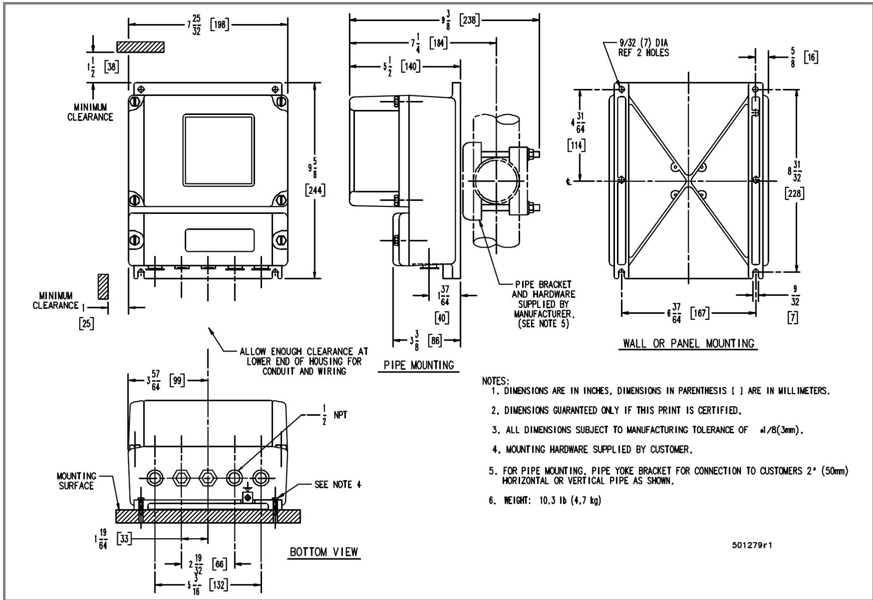
**FIGURE 2-1. OUTLINE DIMENSIONS, REMOTELY MOUNTED 50XM1000N SIGNAL CONVERTER WITH FIXED-COVER & 1/2 INCH NPT CONNECTIONS**
