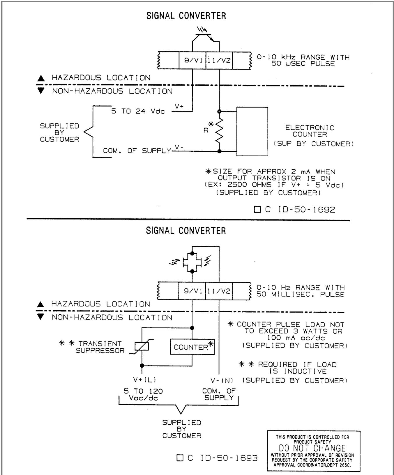
**FIGURE 2-15. INTERCONNECTION WIRING DIAGRAM; SCALER ASSEMBLY**
