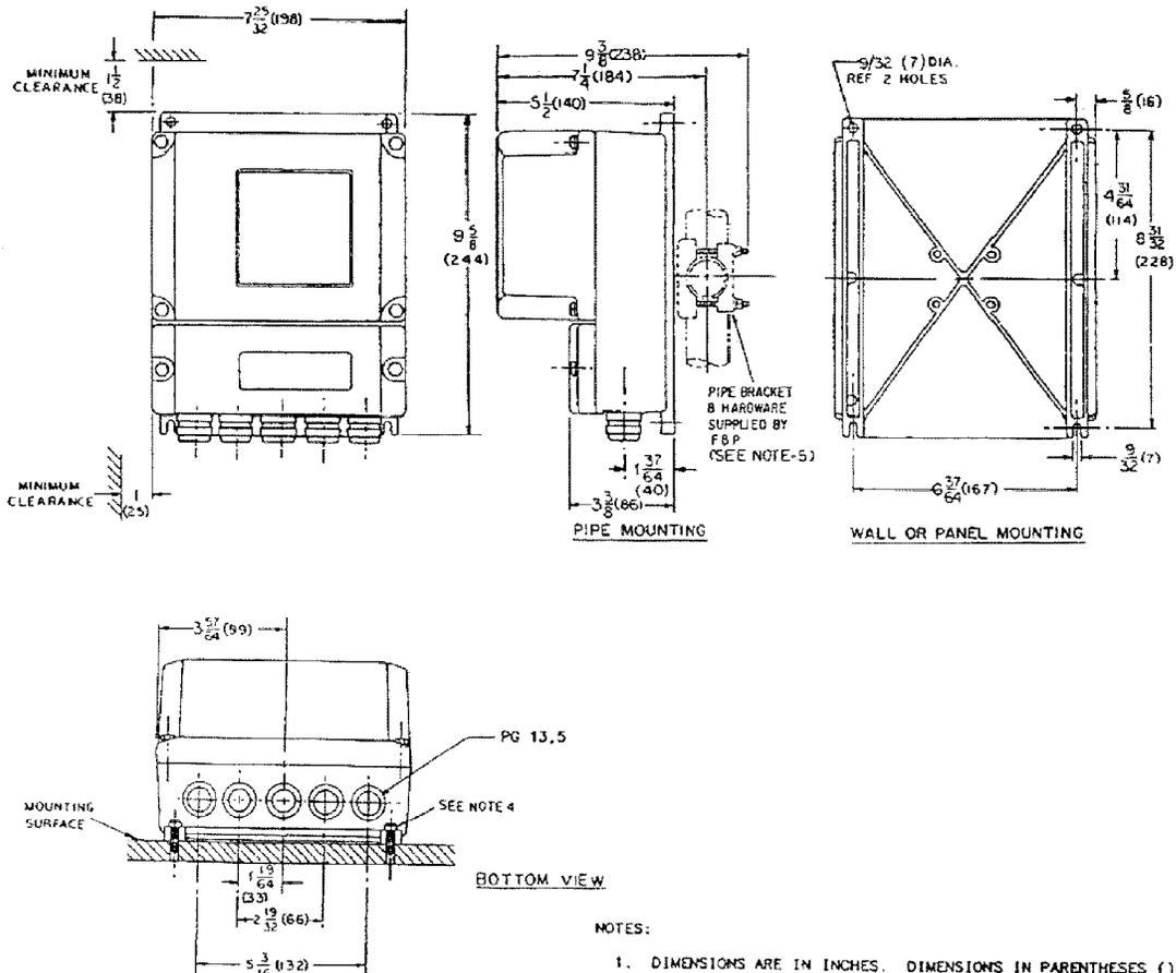
FIGURE 2-2. OUTLINE DIMENSIONS, REMOTELY MOUNTED SIGNAL CONVERTER WITH FIXED-COVER & CABLE SEAL CONNECTIONS
