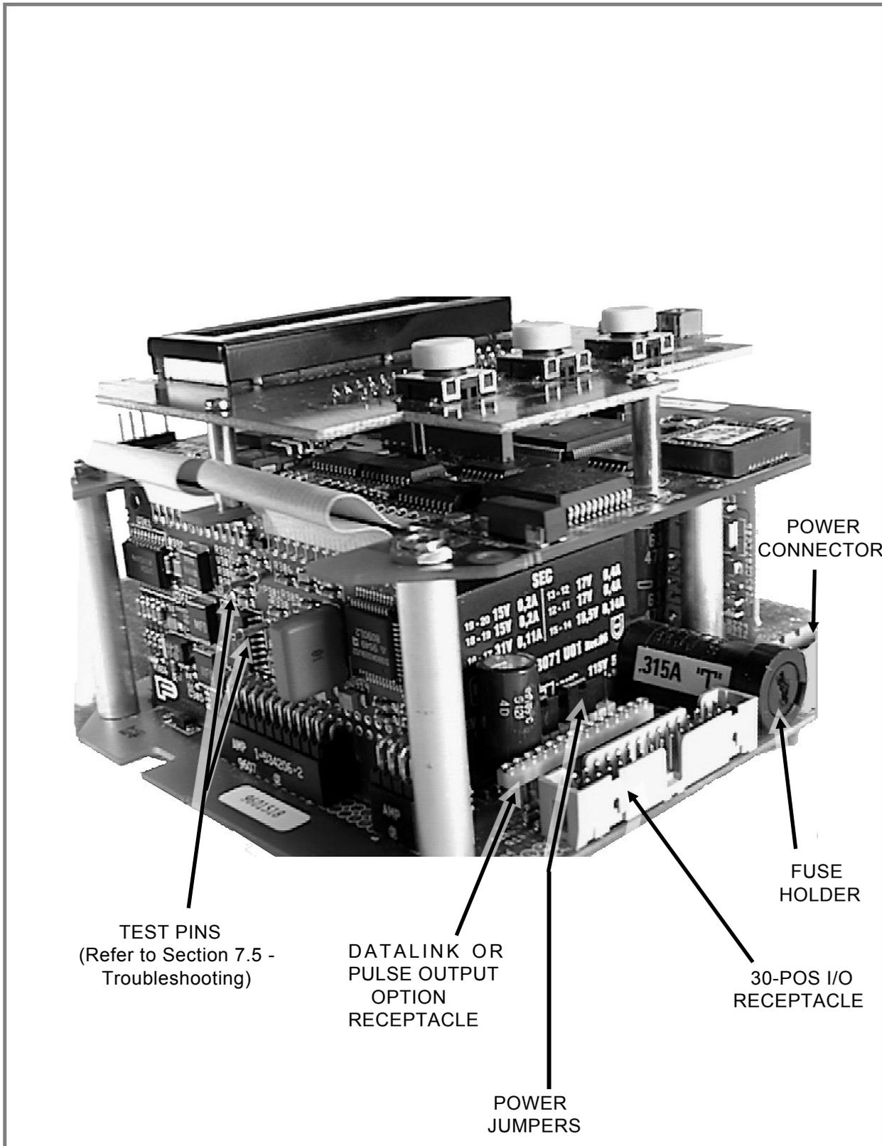
FIGURE 1-4. SIGNAL CONVERTER, SIDE VIEW
