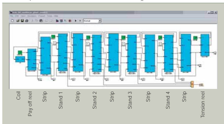
3 Modular process model for a four-stand tandem cold rolling mill
