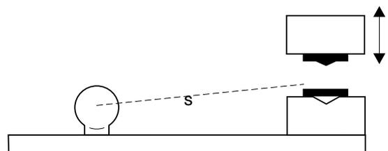
The safety distance is the distance between the Safeballs™ and the dangerous machine movement. Note that S must never be less than 100 mm.
