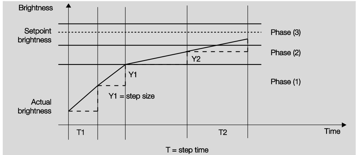
In the start-up phase (1), the *Step time for fast approach* ( $T_1$ ) of the control step can be parameterized. The smaller this time, the faster the control steps are sent with the calculated step increment ( $Y_1$ ). The setpoint brightness is approached in a relatively short time.
