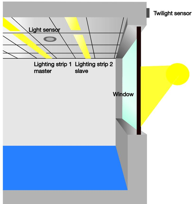
Using the additional function *Slave*, a second lighting strip (slave) can be controlled in the room. Up to now, both lighting strips were normally controlled with the same brightness value.
