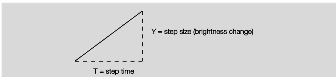
A simplified lighting control can in principle look as follows. The setpoint brightness is achieved starting from an actual brightness level in three steps:
