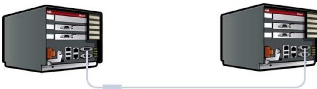
Fig. 6 Serial 1 to serial 1 Redundant link connections with ferrite core
