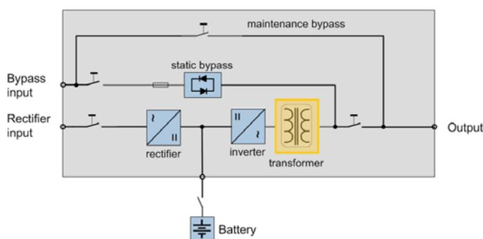
Figure 1: single-line diagram of a transformer-based UPS
