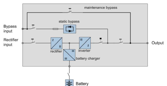
Figure 2: single-line diagram of a transformer-free UPS
