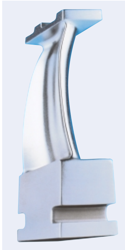
High-performance blade with profile twist and lean to take account of non-uniform flow and pressure distribution over the blade height [8]
