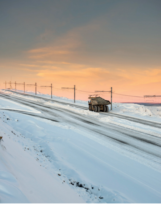
The world's first electric trolley in an Arctic climate at Boliden's Aitik openpit mine
