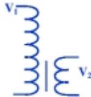
A Symbol of a Potential Transformer
