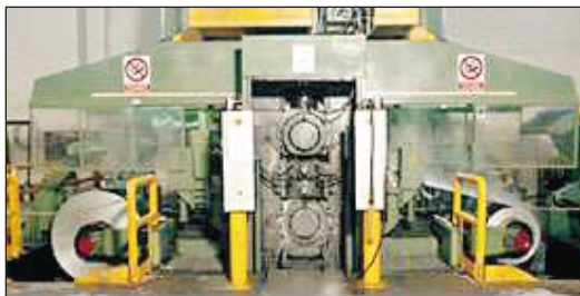
Left: The Cold Rolling Mill at Profilglass in Italy before revamping the thickness gauging systems in 2002 (Strip width 800 mm, min. strip thickness 0.2 mm).
