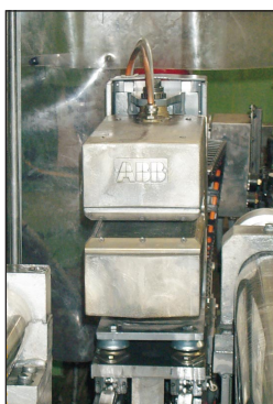
Right and below: In January 2002 the new ABB gauge was installed on the right-hand side of the stand.
