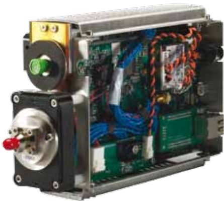
Axsun Tunable Laser – IntegraSpec XLP MEMS NIR Spectrometer Module
