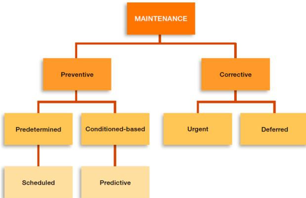
Corrective Maintenance, also known as run-to-failure, assumes that all failures are age-related and inevitable. As the name suggests, no maintenance actions are carried out on the equipment. Upon failure, corrective actions such as repairs or replacements are made. This maintenance strategy should only be applied to equipment with negligible failure consequences.
