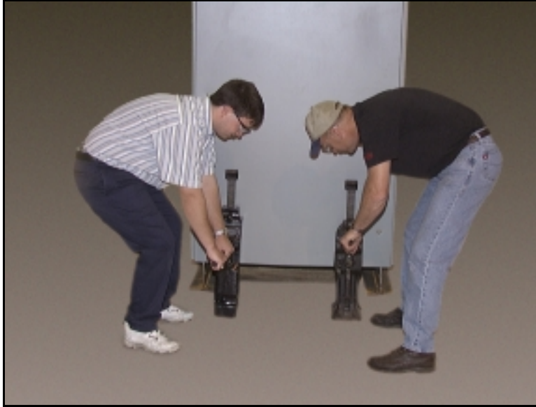
Figure 2: Position jacks under the front and rear corners.
