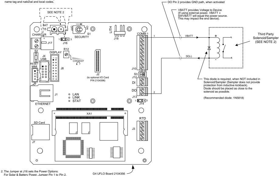
For External Power Source: Jumper Pin 2 to Pin 3.
