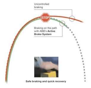
**Collision detection** is especially important on robots of this size. Thanks to this feature, collision forces can be reduced by 70%, improving safety, protecting peripheral equipment and cutting robot downtime in the process.
