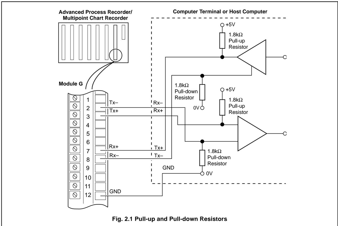
**Fig. 2.1 Pull-up and Pull-down Resistors**
