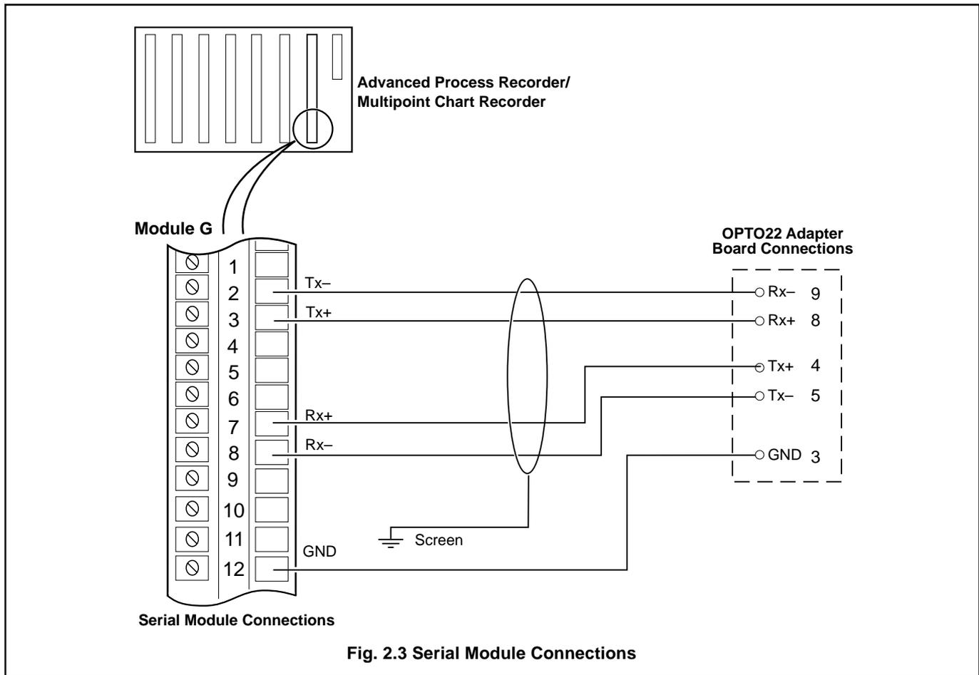
Fig. 2.3 Serial Module Connections
