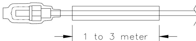
**Figure 10-4. Shrinkable tubing on the cable jacket**
