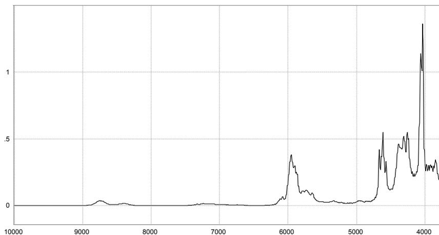
**Figure 3-6. Liquid toluene NIR-absorbance spectrum**
