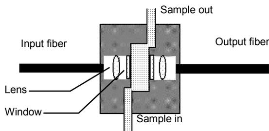
**Figure 8-2. Flow-through cell**
