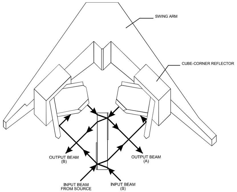
Figure 1-2. Michelson interferometer
