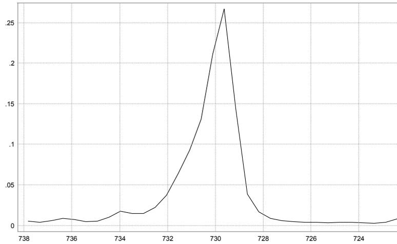
**Figure 4-2. Peak absorbance for acetylene (40 ppm in N<sub>2</sub> at 1 atm.)**
