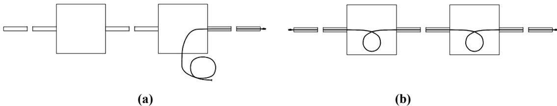
**Figure 10-7.** Pulling fiber-optic cable through conduit
