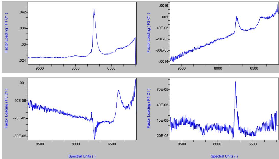
Figure 6-6. PCA factors for modeling fiber-optic behaviour above the OH band
