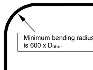
**Figure 10-2. Minimum bending radius for fiber-optic cables**
