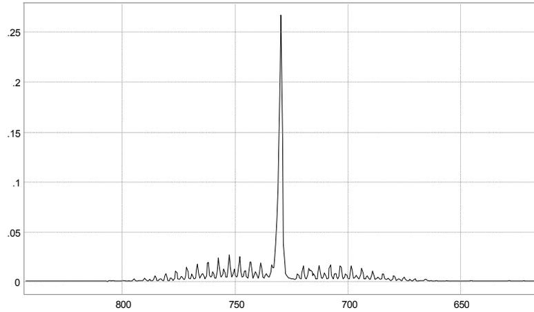
**Figure 4-1. Acetylene absorbance spectrum (40 ppm in N<sub>2</sub> at 1 atm.)**
