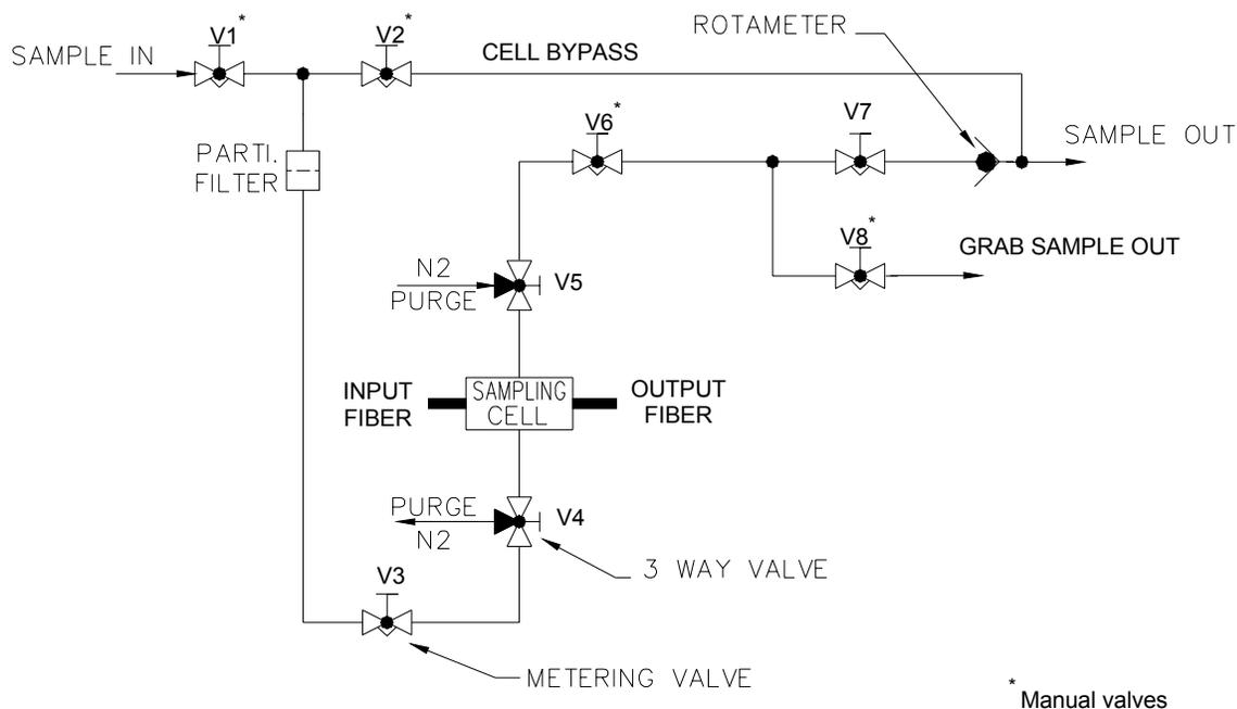
**Figure 8-4. Sampling system for a flow-through cell**
