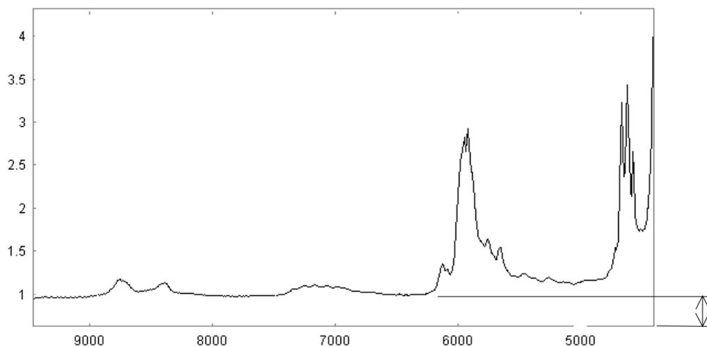
**Figure 8-5. Signal loss due to air bubbles**
