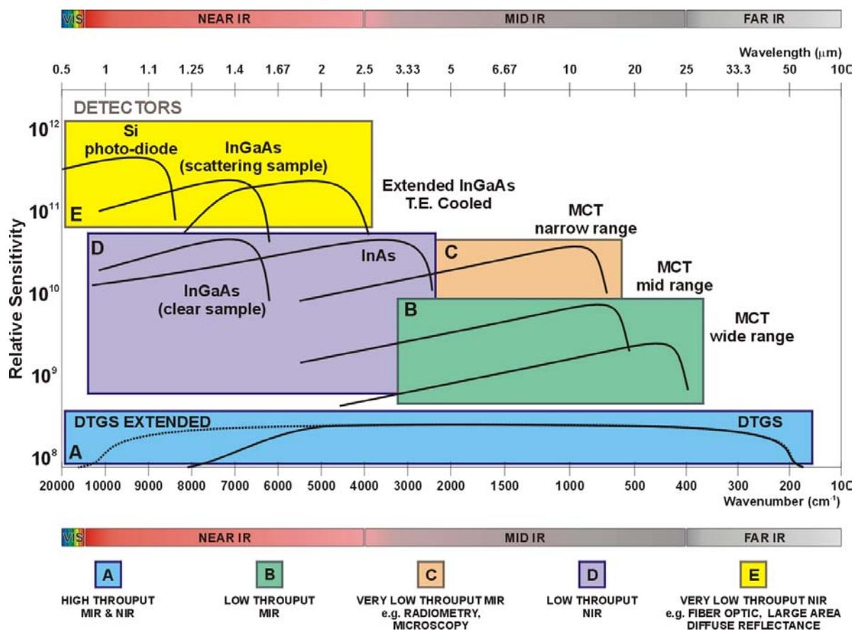
Figure A-1. Spectral characteristics of different detectors
