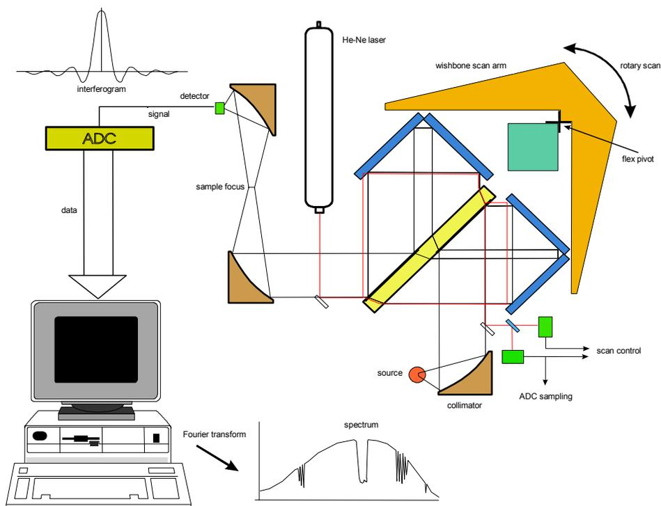
Figure 3-7. Operating principle
