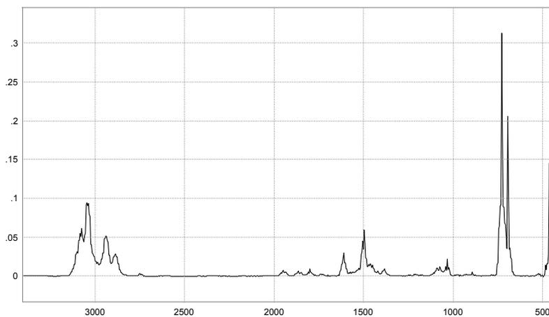
Figure 3-5. Toluene vapor MIR-absorbance spectrum (500 ppm in  $\text{N}_2$  at 1 atm.)<sup>f</sup>
