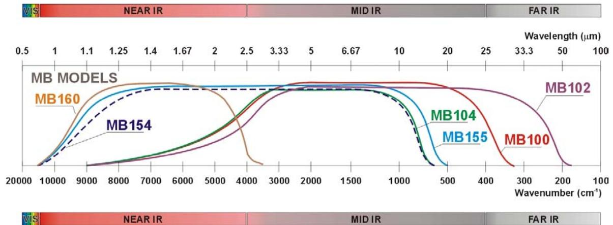
Figure A-2. Spectral characteristics of different MB Series Spectrometer models
