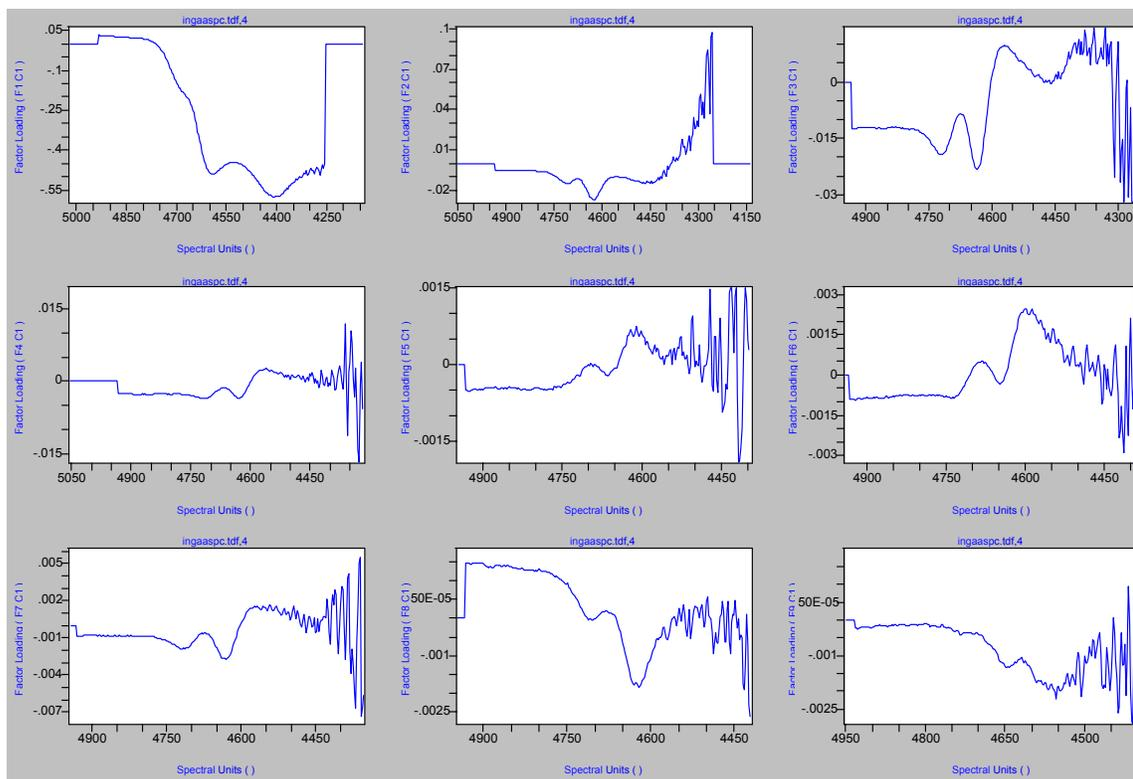
**Figure 6-3. PCA factors in an attempt to model detector behaviour below 4200 cm<sup>-1</sup>**
