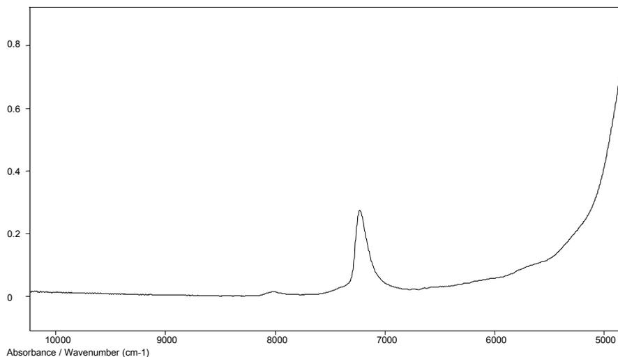
**Figure 6-4. Spectral response of a 100-m fiber-optic cable**
