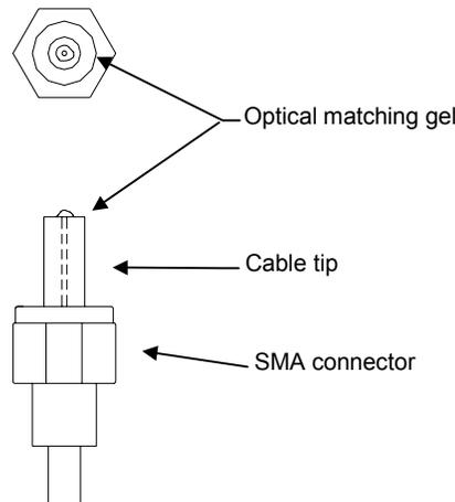
**Figure 10-8. Optical matching gel on cable tip and matching connector**
