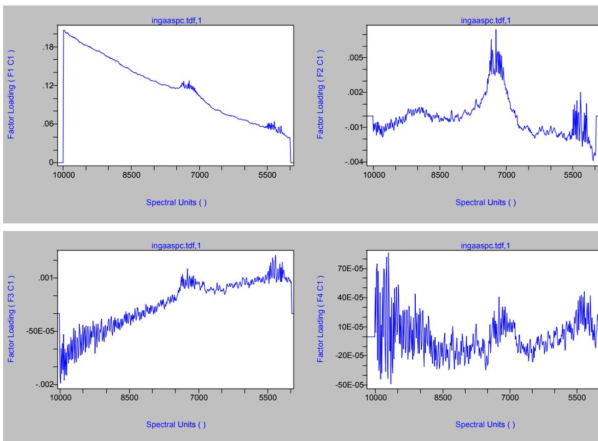
**Figure 6-2. PCA factors for modeling detector behaviour above  $5000\text{ cm}^{-1}$**
