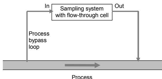
**Figure 8-1. Process bypass loop**
