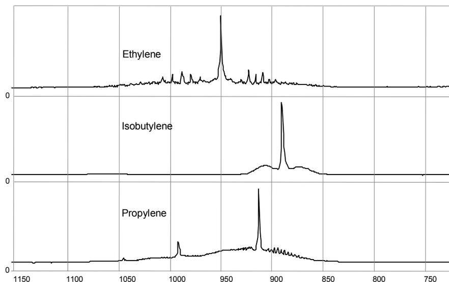
**Figure 4-5. Chemical and spectral signature**
