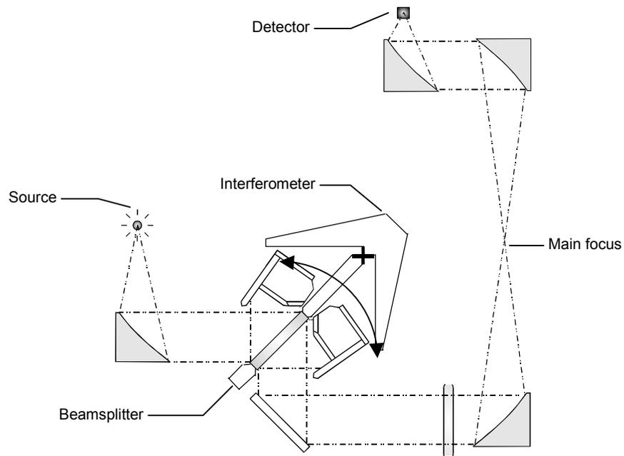
**Figure 1-1. Schematic diagram of ABB spectrometers**
