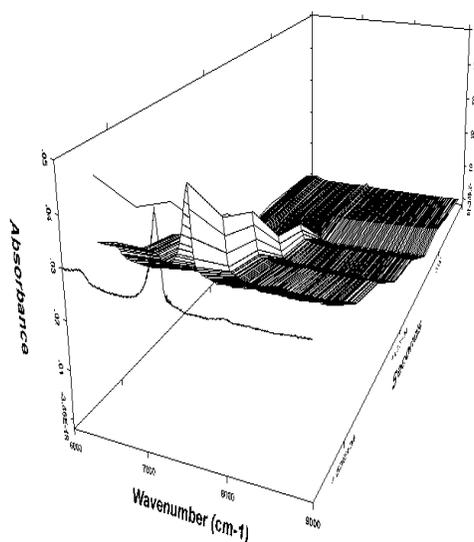
**Figure 6-5. Spectral response of an optical fiber as temperature is varied**
