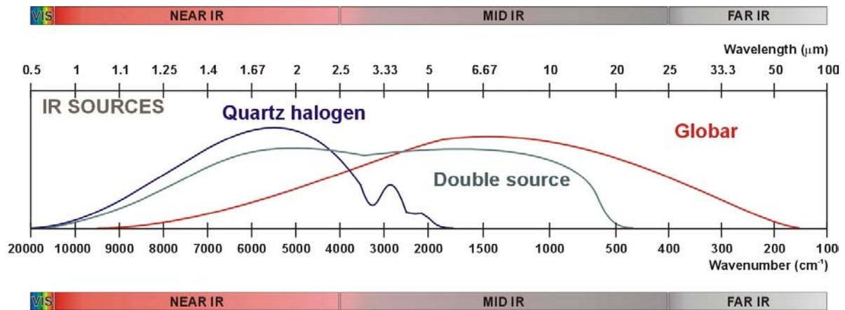
Figure A-3. Spectral characteristics of different IR sources
