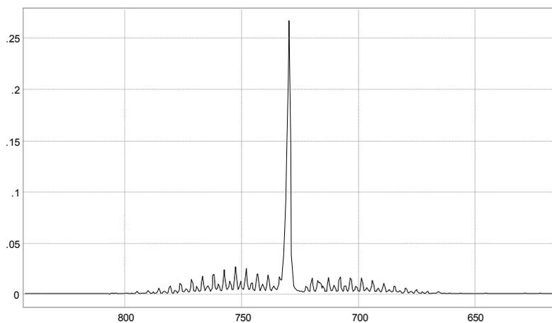
Figure 3-4. Acetylene absorbance spectrum (40 ppm in  $\text{N}_2$  at 1 atm.)<sup>e</sup>
