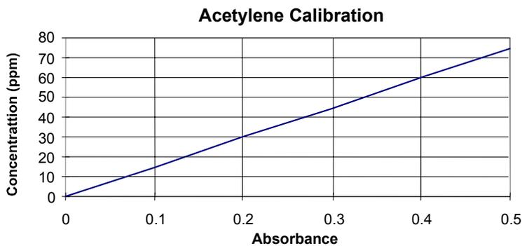
Figure 4-3. Peak-height calibration plot
