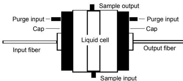
**Figure 8-6. Flow-through cell with purge caps**
