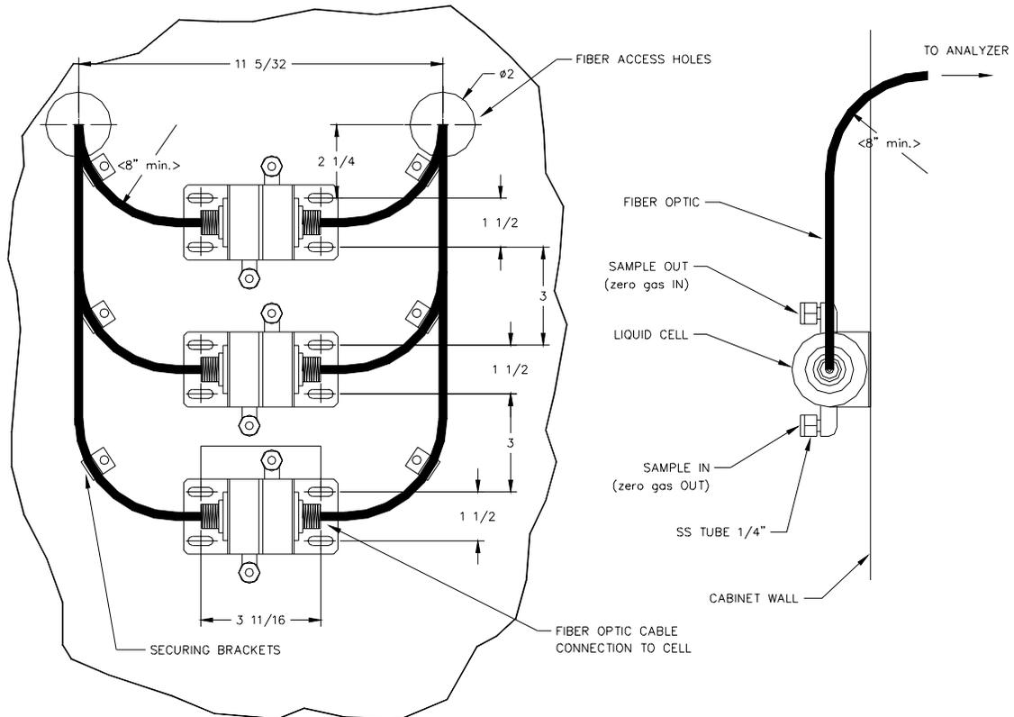
**Figure 8-3. Installation of flow-through cells**
