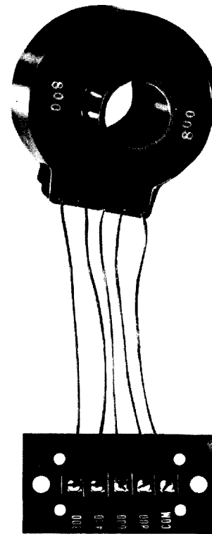
Figure 2-1 MicroVersaTrip® RMS-9 Phase Sensor
