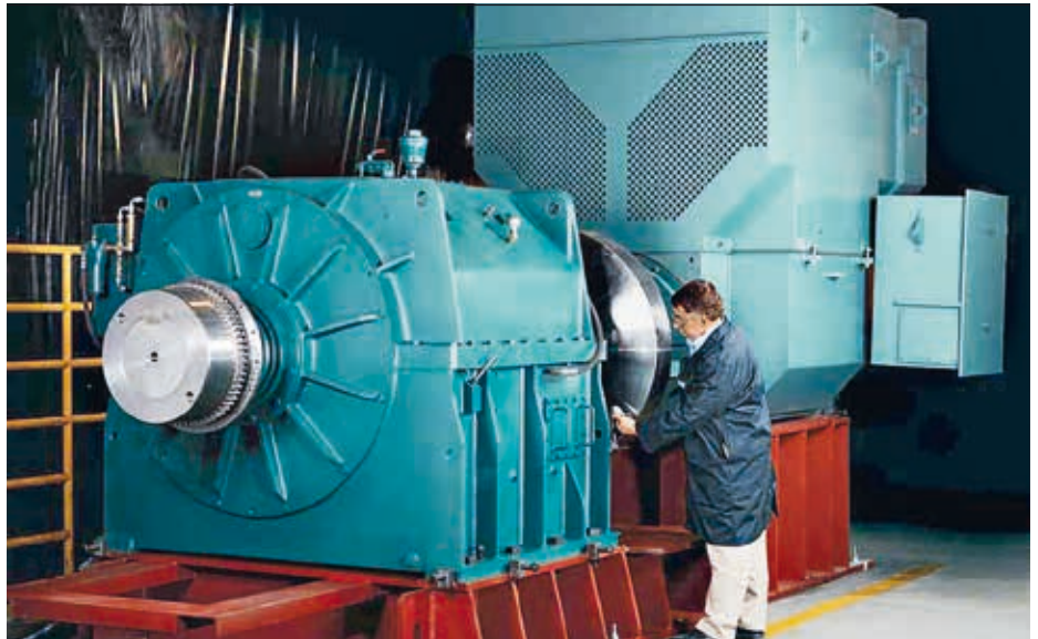
1 Fully assembled drive system package featuring a 2,500 K Dodge CST, a 2,500 hp Baldor Reliance motor, an optional 3,150 pound fly-wheel and high- and low-speed couplings
