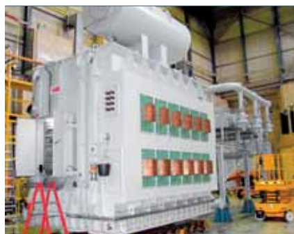
9 An air-cooled rectifier transformer rated 91.74 MVA
