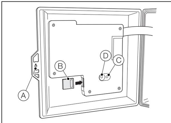
Fig. 9.13 SD card insertion / removal
