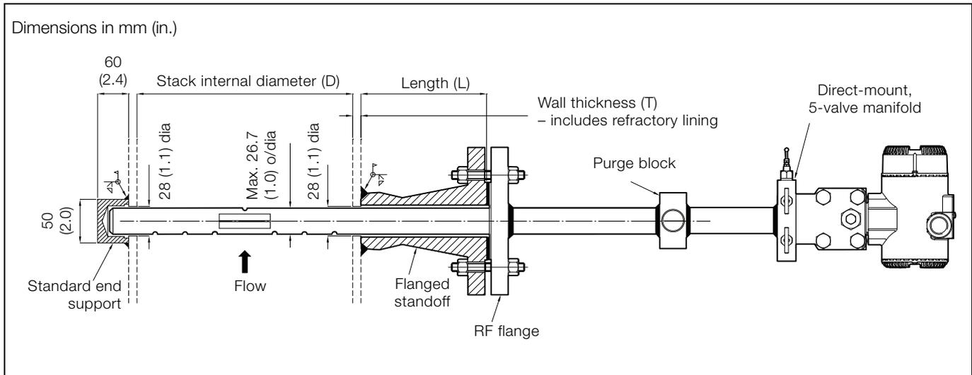
3.2.3 Probe – 25 mm (1.0 in.) diameter with flanged end support (with integral transmitter)
