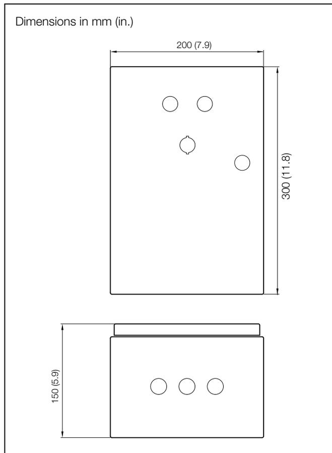
Fig. 4.1 FPD583 manual interface unit dimensions
