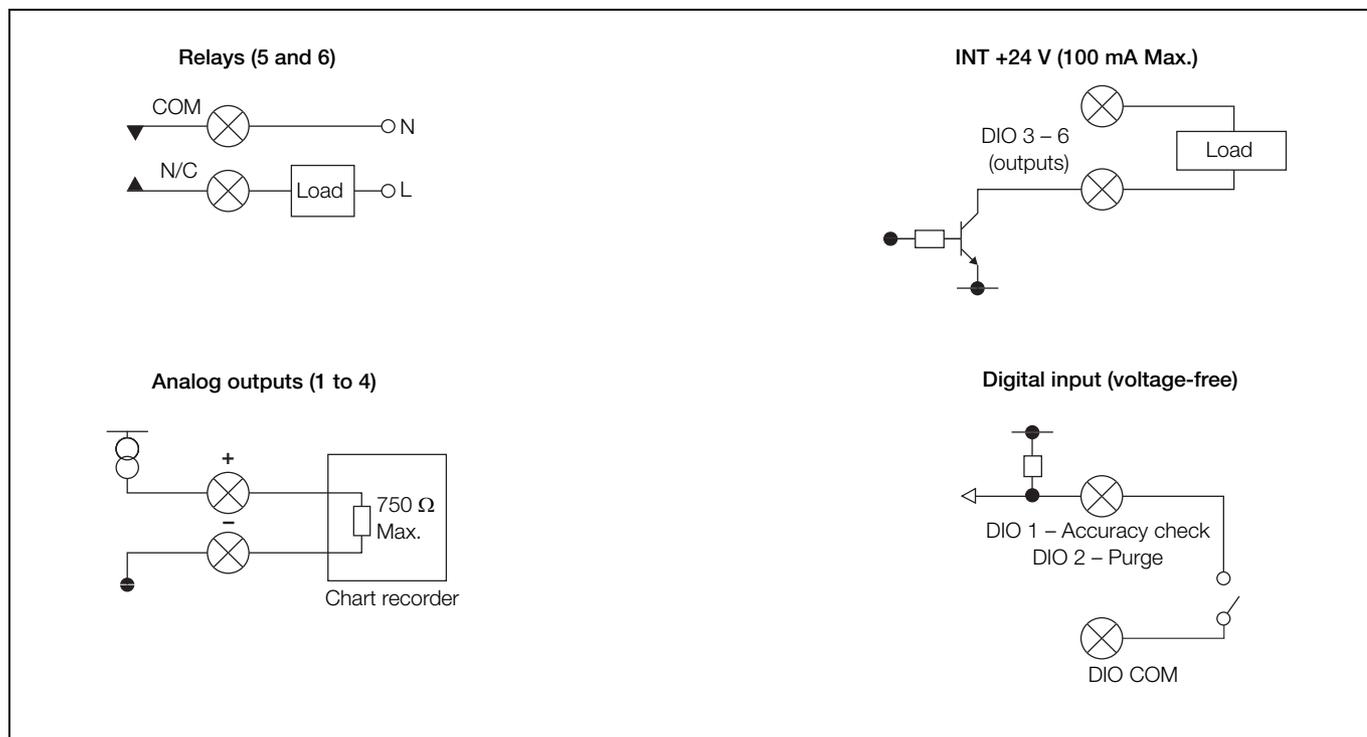
Fig. 5.3 Digital I/O, relay and analog output connections
