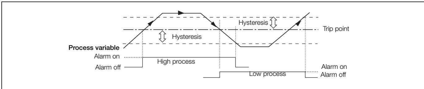
Fig. 9.17 Process alarm example – high and low process alarm action
