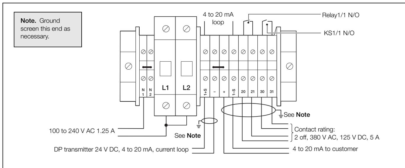
Fig. 5.1 Interface unit A connections
