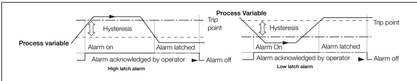
Fig. 9.18 High and low latch alarm action
