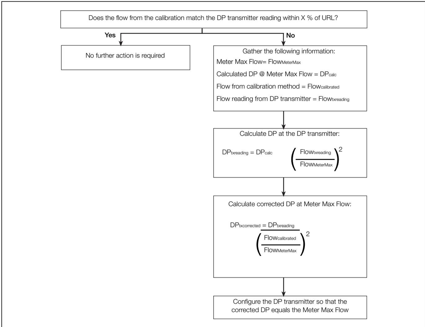
Fig. 7.2 Method to correct DP following calibration
