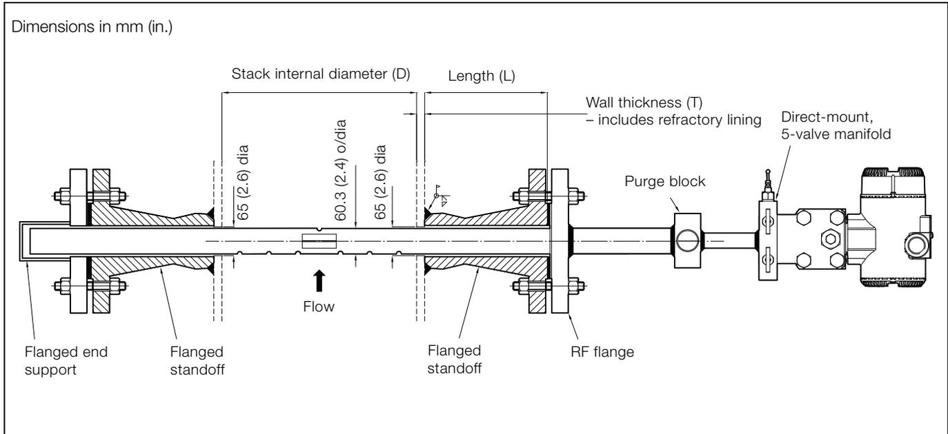
3.2.6 Probe – 60 mm (2.4 in.) diameter with weldcup end support (with integral transmitter)
