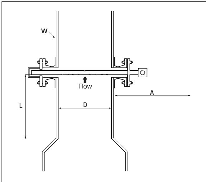
Fig. 3.1 Installation requirements
