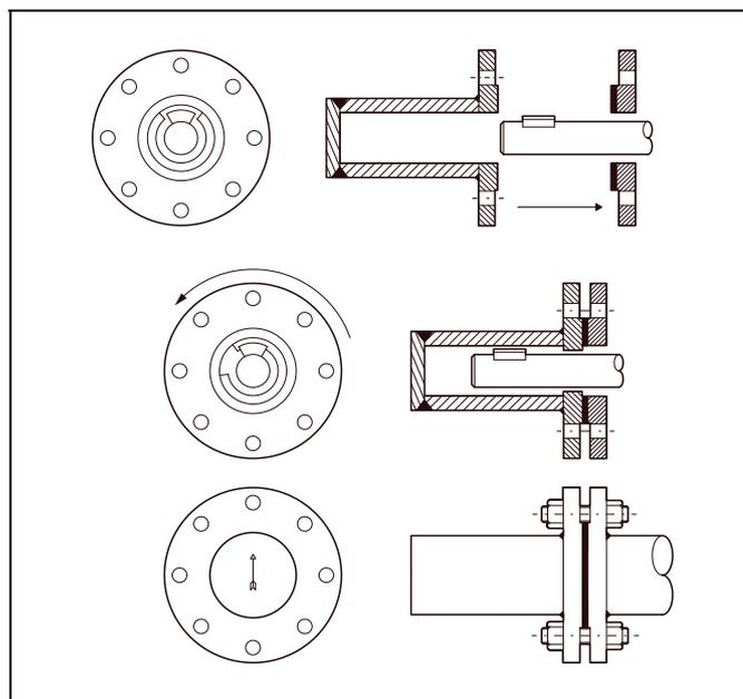
Fig. 3.5 Bayonet fitting installation details
