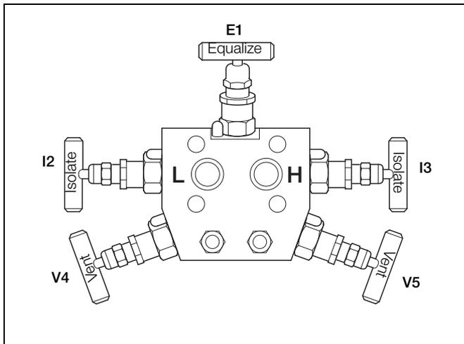
Fig. 7.1 Valve identification (view from underside of manifold)
