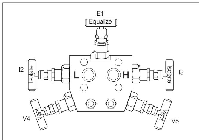
Fig. 10.1 Valve identification (view from underside of manifold)
