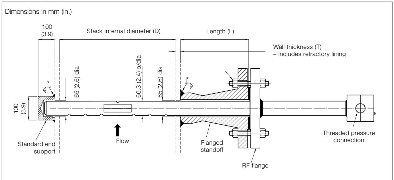
3.2.5 Probe – 60 mm (2.4 in.) diameter with flanged end support (for integral transmitter)
