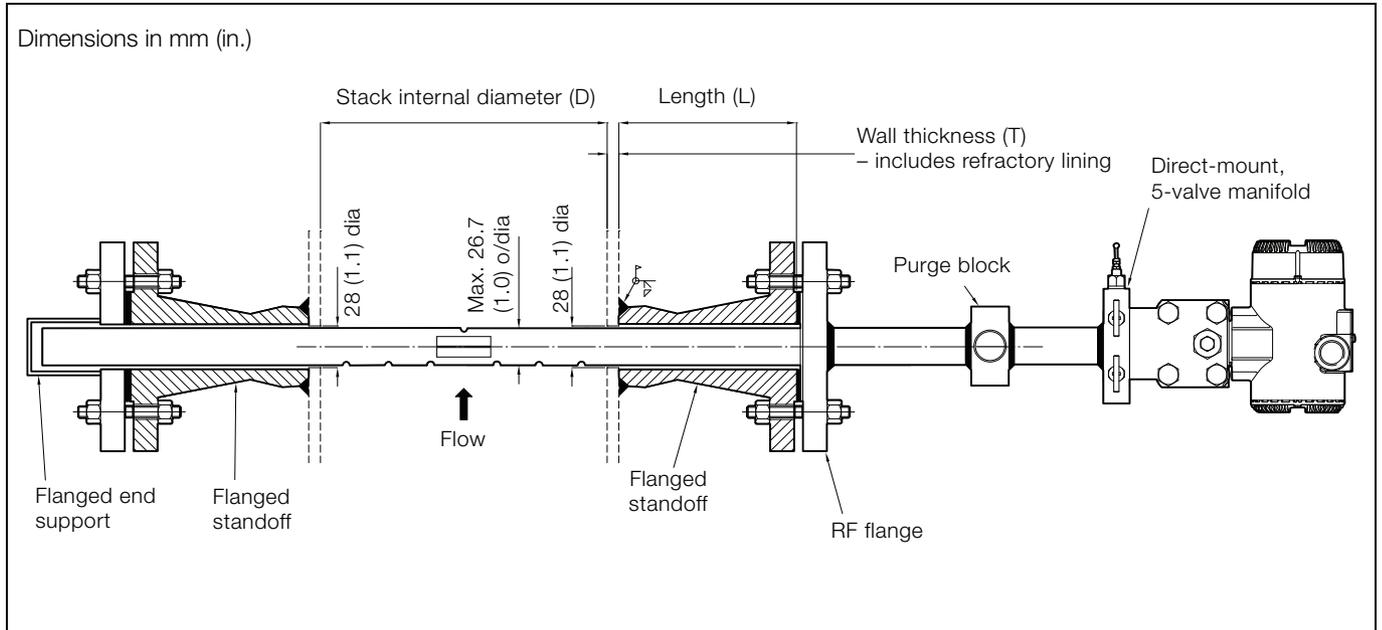
3.2.4 Probe – 60 mm (2.4 in.) diameter with weldcup end support (for remote transmitter)
