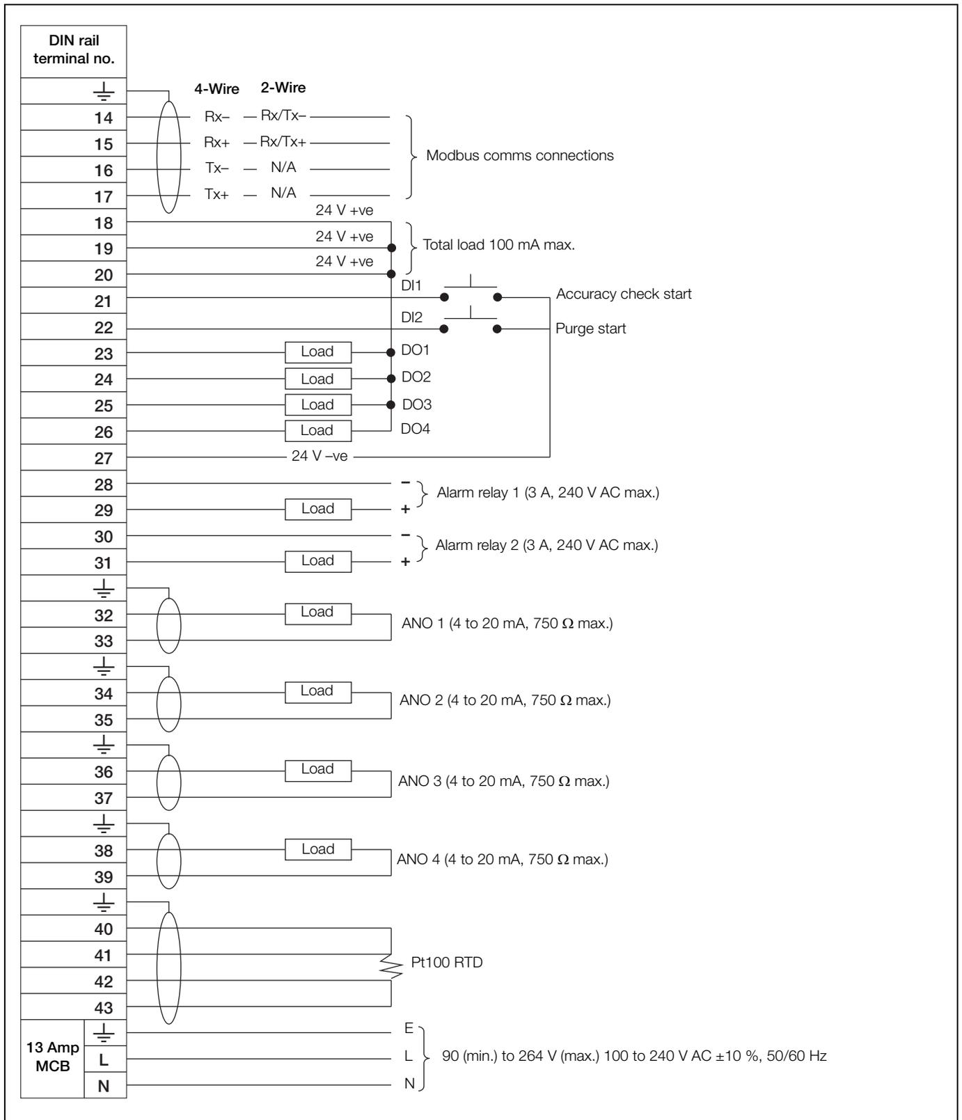
Fig. 5.2 Interface unit B, C and D connections
