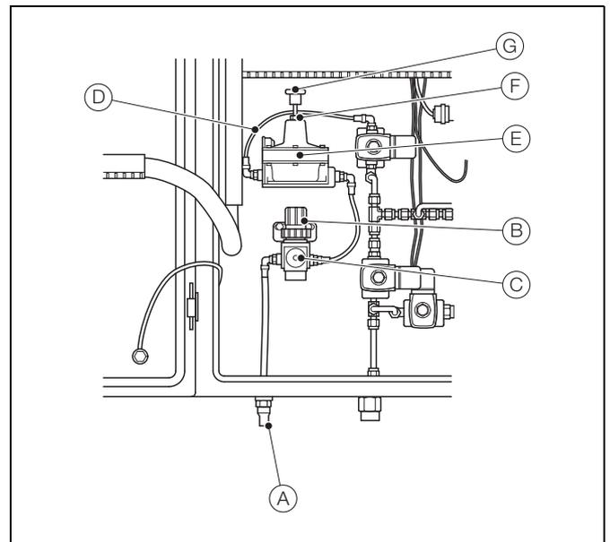
Fig. 10.3 Checking / Setting the span pressure regulator
