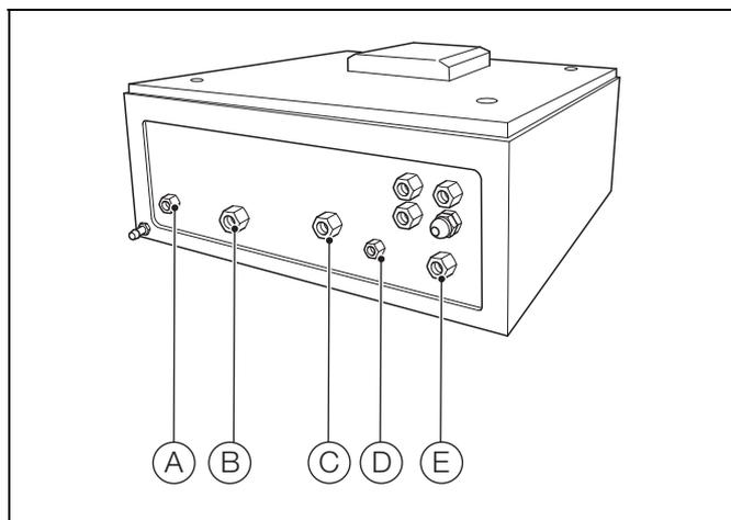
Fig. 6.1 Interface unit B (without auto span check) – pneumatic connections
