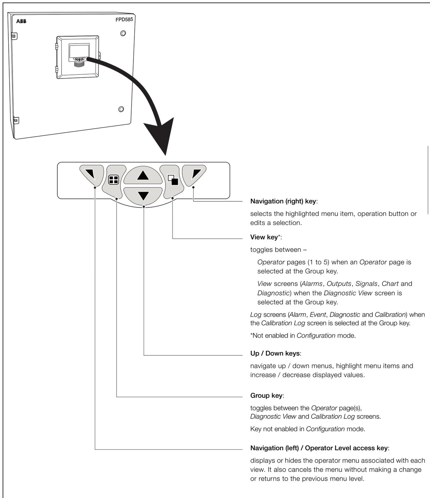
Fig. 9.1 Front panel keys
