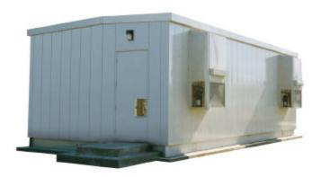
The PDC-4000 is a prefabricated modular, skid-mounted enclosure for switchgear and auxiliary equipment. As a self-contained unit, it is completely coordinated, assembled and tested in controlled factory environment. With integral transformers, close-coupled to switchgear or with bus duct connections, a PDC-4000 can serve as a complete unit substation
