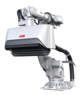
The FeatherDuster system advances vehicle paint lines by replacing purpose-built "tack off" machines with robotic technology that is incredibly flexible and built on well-established standards to achieve higher quality, efficiency and ease of use.
