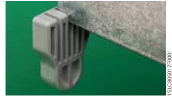
The fixing hooks and feet supplied in the standard versions are applied without having to use tools, making it possible to install the base plate at seven different depths inside the switchboard. They can also be adjusted at three further positions.
