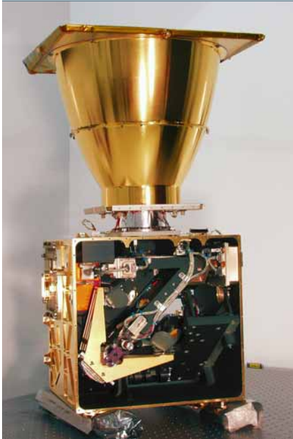
2 The Canadian Space Agency's SciSat satellite is equipped with the ABB ACE-FTS (Atmospheric Chemistry Experiment – Fourier Transform Spectrometer) instrument
