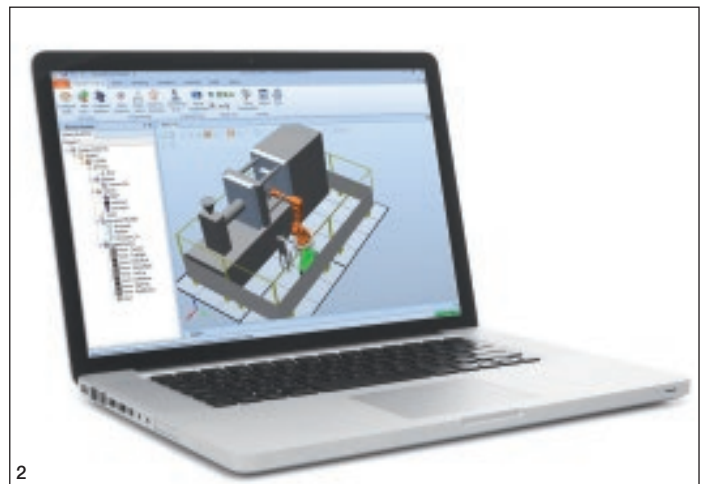
1. ABB's FlexPendant operator device has an intuitive graphical user interface that is fully customizable to the user's requirements. | 2. RobotStudio is a graphical programming environment that allows robots to be programmed offline, reducing downtime while minimizing the risk of programming error.
