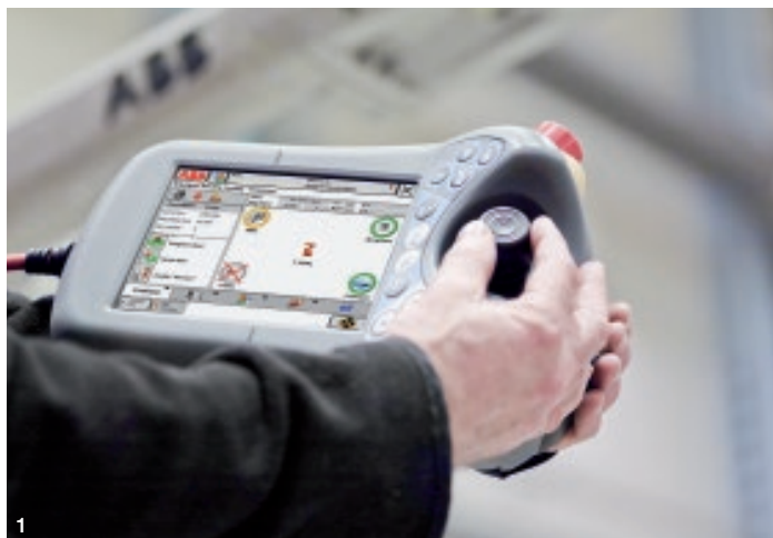
1. ABB's FlexPendant operator device has an intuitive graphical user interface that is fully customizable to the user's requirements. | 2. RobotStudio is a graphical programming environment that allows robots to be programmed offline, reducing downtime while minimizing the risk of programming error.
