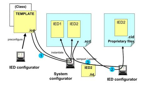
Figure 3. Modification process [IEC09].
