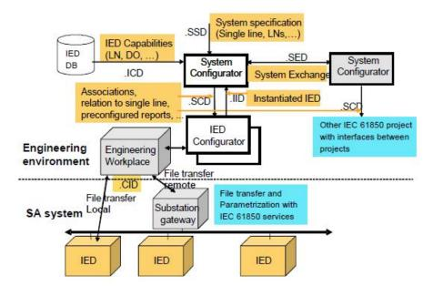
Figure 2. Reference model for the information flow in the configuration process [IEC09].
