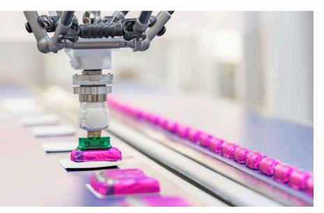
One Conveyor Tracking Module (CTM module) has connections for up to 4 robots, 4 conveyors and 8 cameras. This not only reduces field wiring by 60%, but also reduces the total integration costs and streamlines installation
