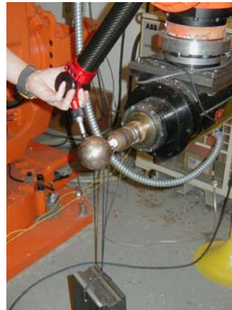
Figure 4: Experiment Setup of robot stiffness measurement
