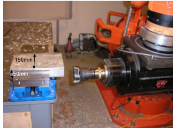
Figure 9: Experimental setup for robotic milling
