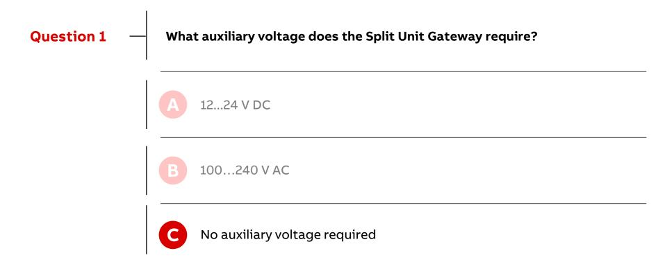
Supply voltage via ABB i-bus KNX
