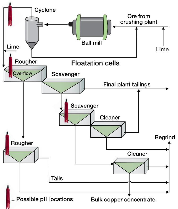
The pH sensor in any mineral processing slurry should be mounted to provide sufficient velocity past the sensor to minimize lime scale and material buildup. However, the location must trade off flow
