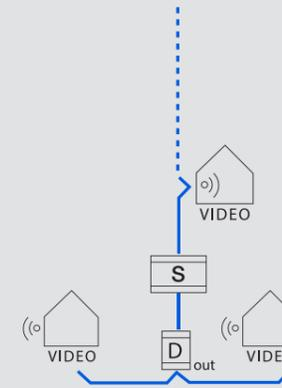
2. 2 level cascading connection for 3 outdoor stations with outdoor distributor
