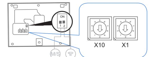
**Setting of the system controller working mode "One on" or "All on"** Fig.103
