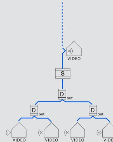
3 level cascading connection for 8 outdoor stations with outdoor distributor
