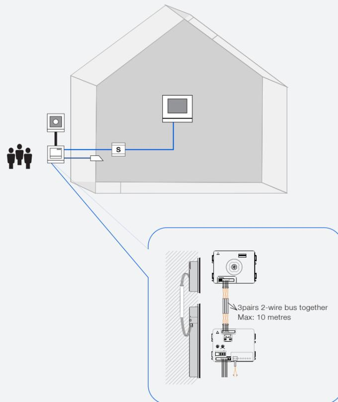
2.6 Power consumer and distance calculation to an insulated system of Welcome system
