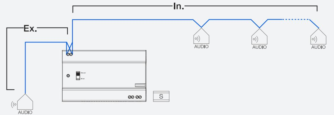
Internal bus and external bus in networked system
