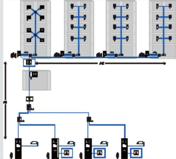
One standard system controller is not enough, and distance is problem, need to add a local power supply for each outdoor station and a gateway in the internal bus of common part.
