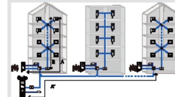
B: The distance from system controller to the furthest indoor station (Table 2-1)
