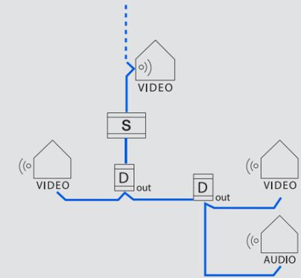
2 level cascading connection for 4 outdoor stations with outdoor distributor
