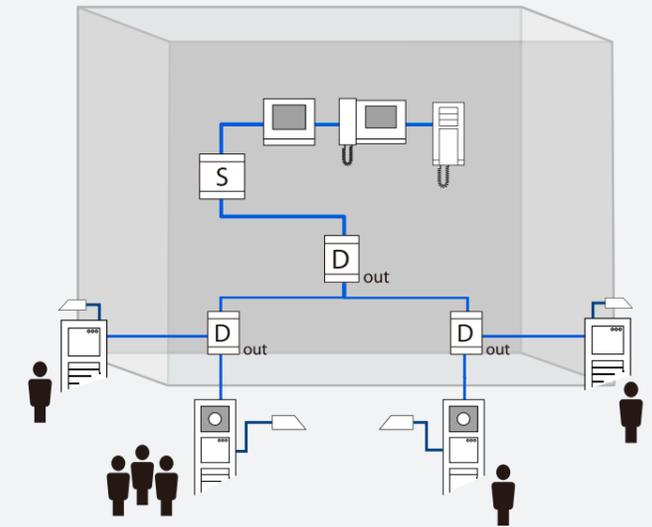
The drawing shows the easy-to-install 2-wire bus connect indoor stations and multi outdoor stations. The outdoor distributor is needed to connect the multi outdoor stations together.
