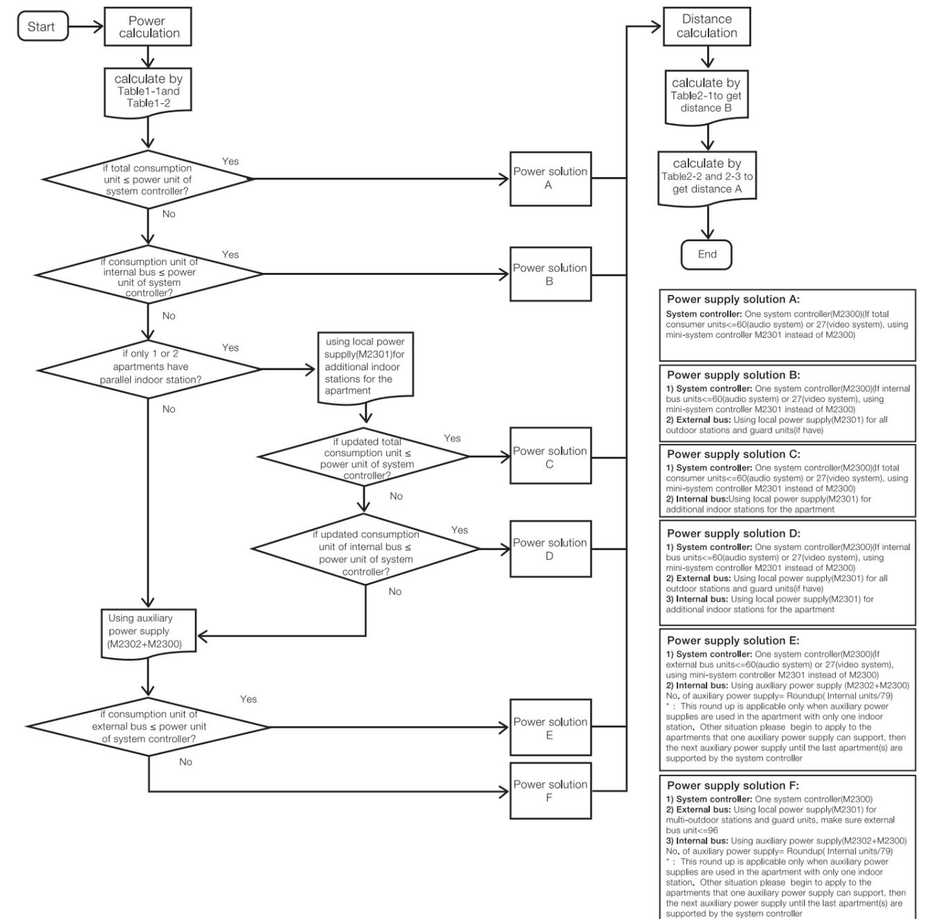
**Table 1-1: Power consumer calculation & attenuation unit (system controller)**
