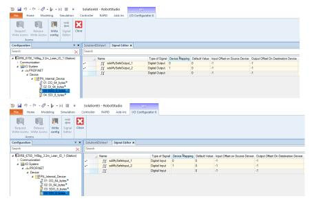
When signal configuration is completed, you can write the configuration to the controller from the I/O Engineering tool or from Visual SafeMove.
