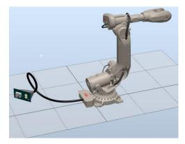
Note that you need to Disconnect the simulation model from its file first. Then you can move the contactor using e.g. SetPosition or free-hand move. You need to use Selection Level = Part.
