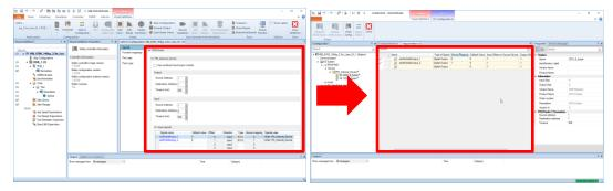
The I/O Engineering Tool can be opened from the Configuration menu of the Controller tab.
