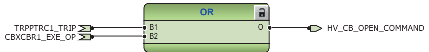
Figure 85: Circuit breaker control logic: Signals for opening coil of high-voltage side circuit breaker
