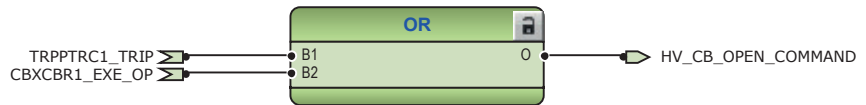
Figure 363: Circuit breaker control logic: Signals for opening coil of high-voltage side circuit breaker
