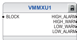
Figure 274: Voltage measurement: Three-phase voltage measurement (HV side)
