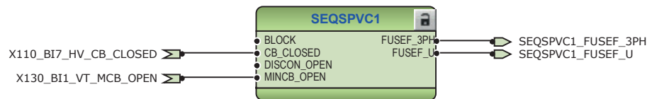
Figure 355: High-voltage side fuse failure supervision function
