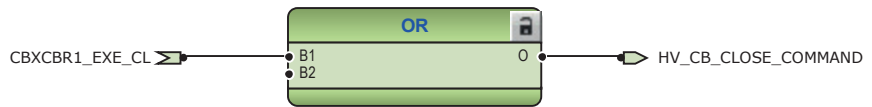
Figure 84: Circuit breaker control logic: Signals for closing coil of high-voltage side circuit breaker
