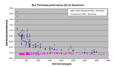
Thickness performance analysis: comparison of customers mill versus benchmark reference plant
