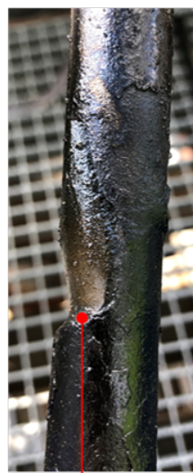
Example of cavitation wear on thermowells
