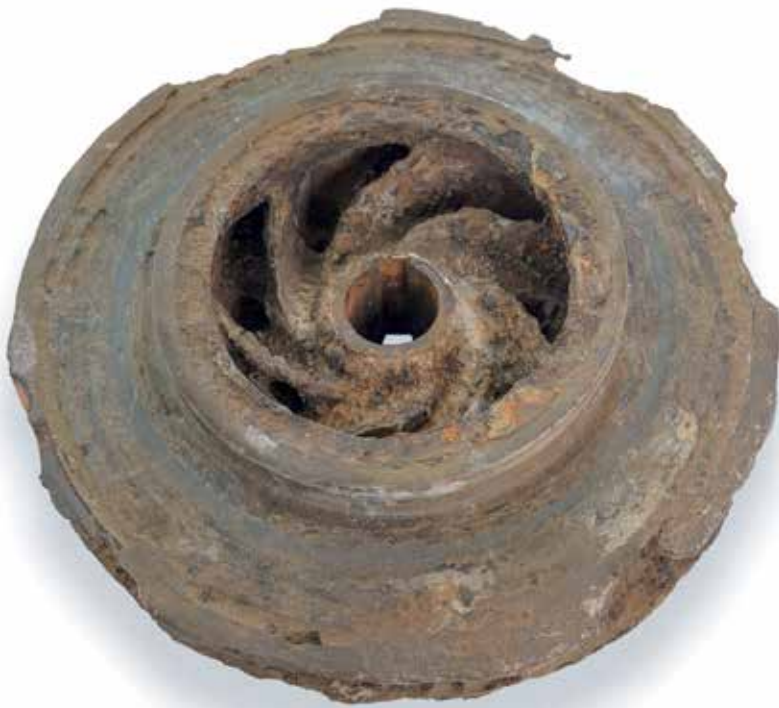
Pump impeller damaged by cavitation
