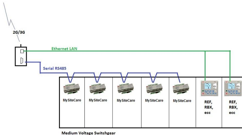
Figure 5: Communication architecture example
