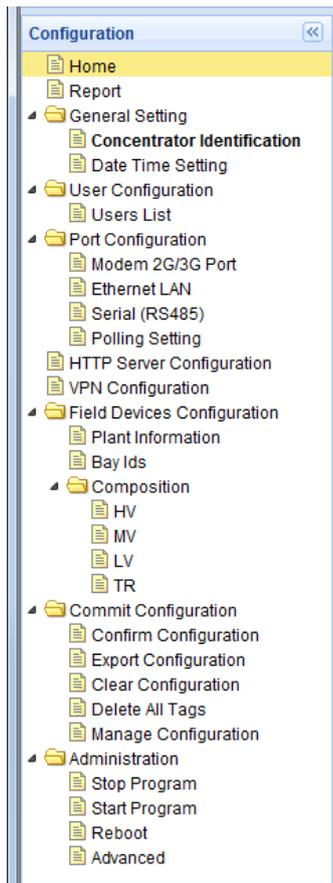
Figure 8: Web HMI Menu Structure
