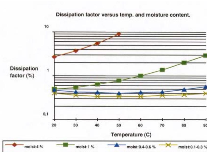
Fig. 1.  $\tan \delta$  as a function of moisture level and temperature on OIP bushings.
