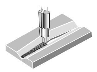
Weldguide IV is a powerful Thru-Arc™ tracking sensor based on patented technology and designed for ABB robotic welding systems.
