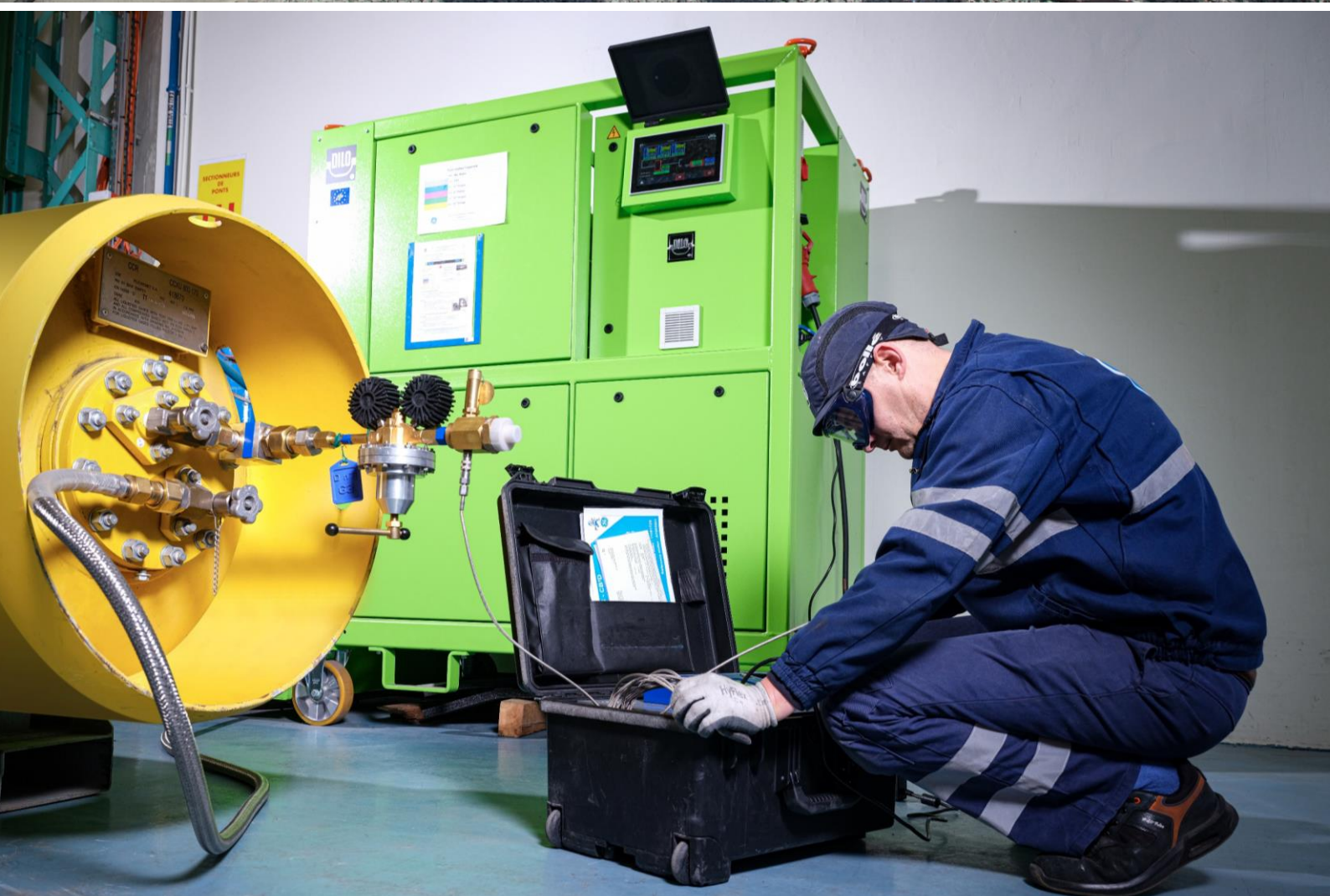
Figure 43: Gas quality routine check of a recently prepared gaseous premixed mixture using a mixing cart
