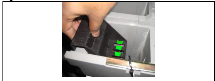
Figure 8.3. Wear Indicator Insertion
