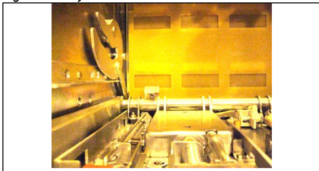
Fig. 5.7. Safety Shutter in Closed Position
