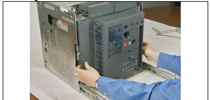
Figure 3.17. Circuit breaker Pulled Out of the Cassette for Unloading
